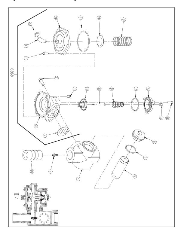
Figure 4-1: Model 52 Pressure Regulator Valve
